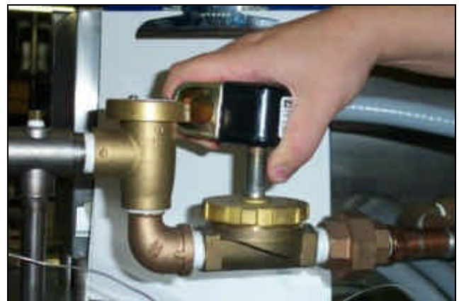
Removing the coil
